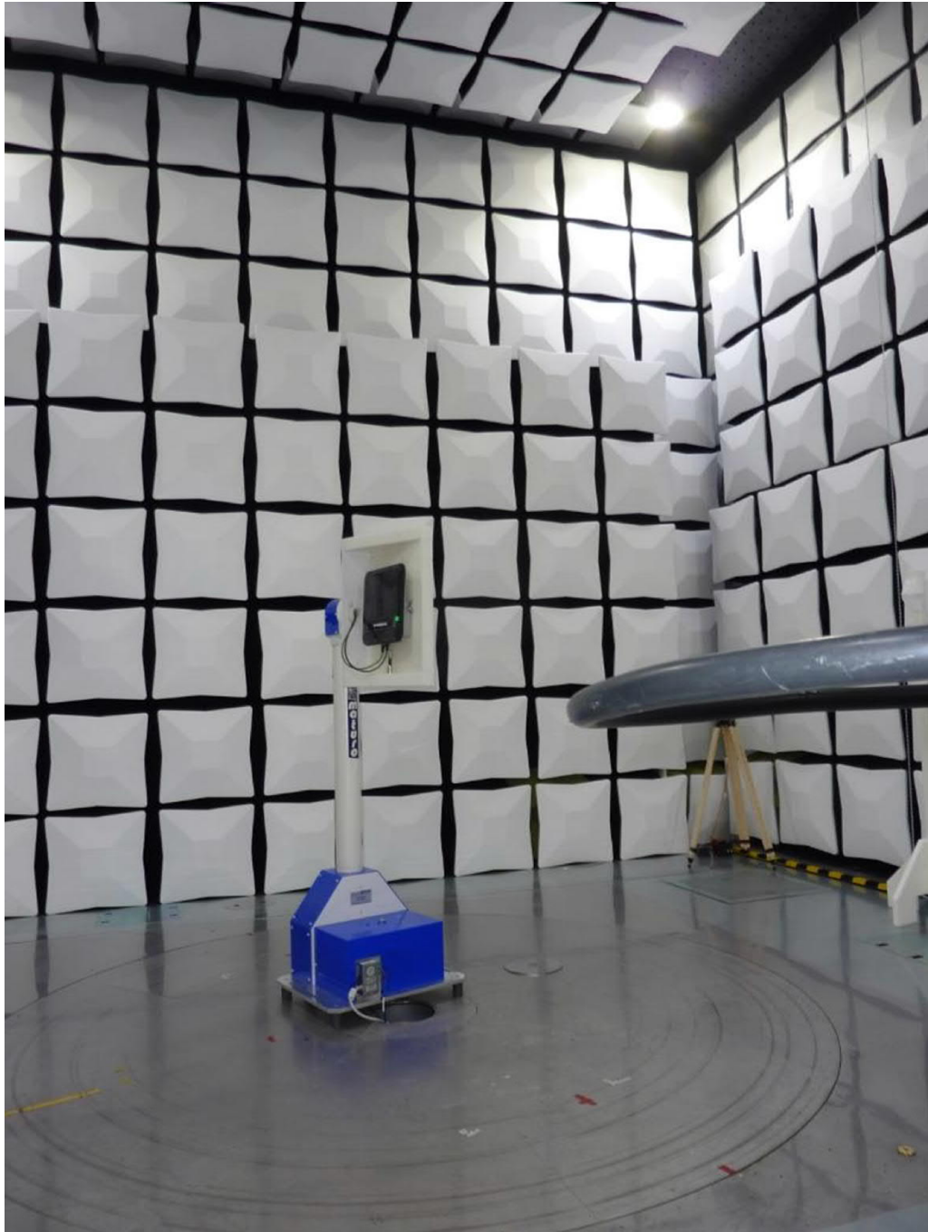
TN-UHF-Q300-NA-CDS, test setup semi anechoic chamber TX spurious emissions from 150 kHz to 30 MHz
