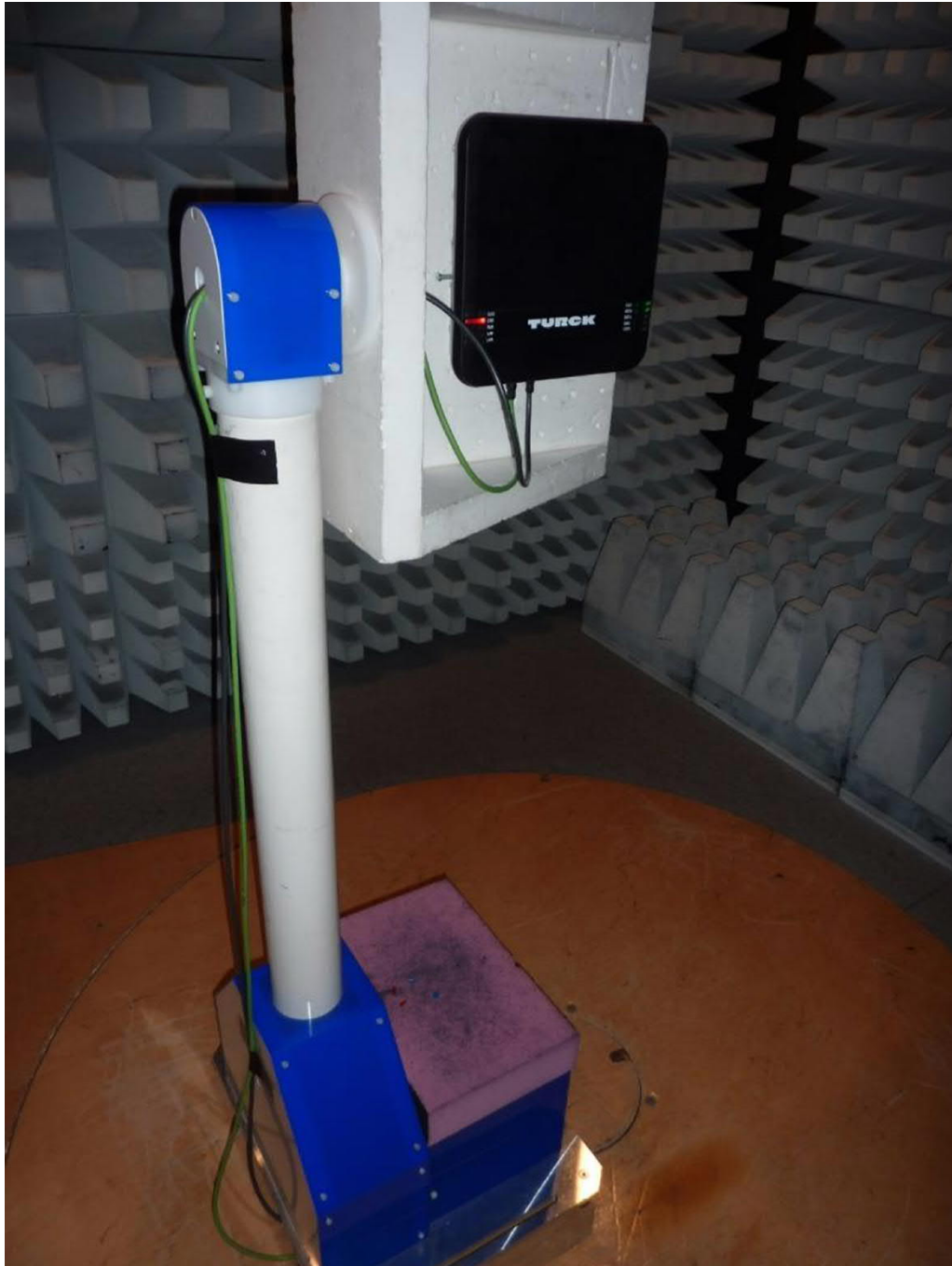
TN-UHF-Q300-NA-CDS, test setup fully anechoic chamber TX spurious emissions from 1 GHz to 10 GHz (measurement with internal antenna)
