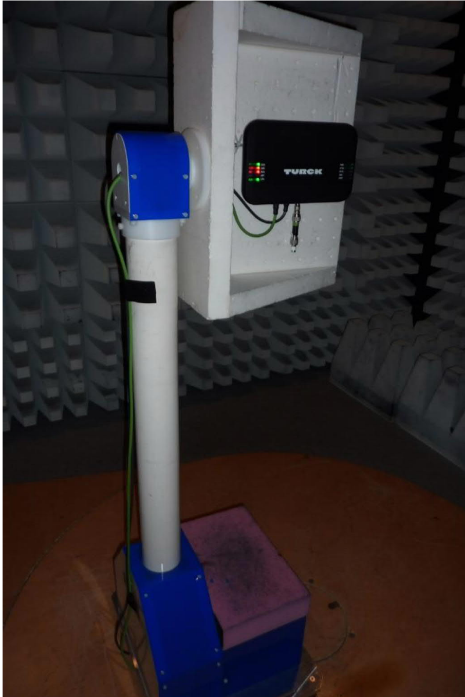
TN-UHF-Q180L300-NA-CDS, test setup fully anechoic chamber TX spurious emissions from 1 GHz to 10 GHz
