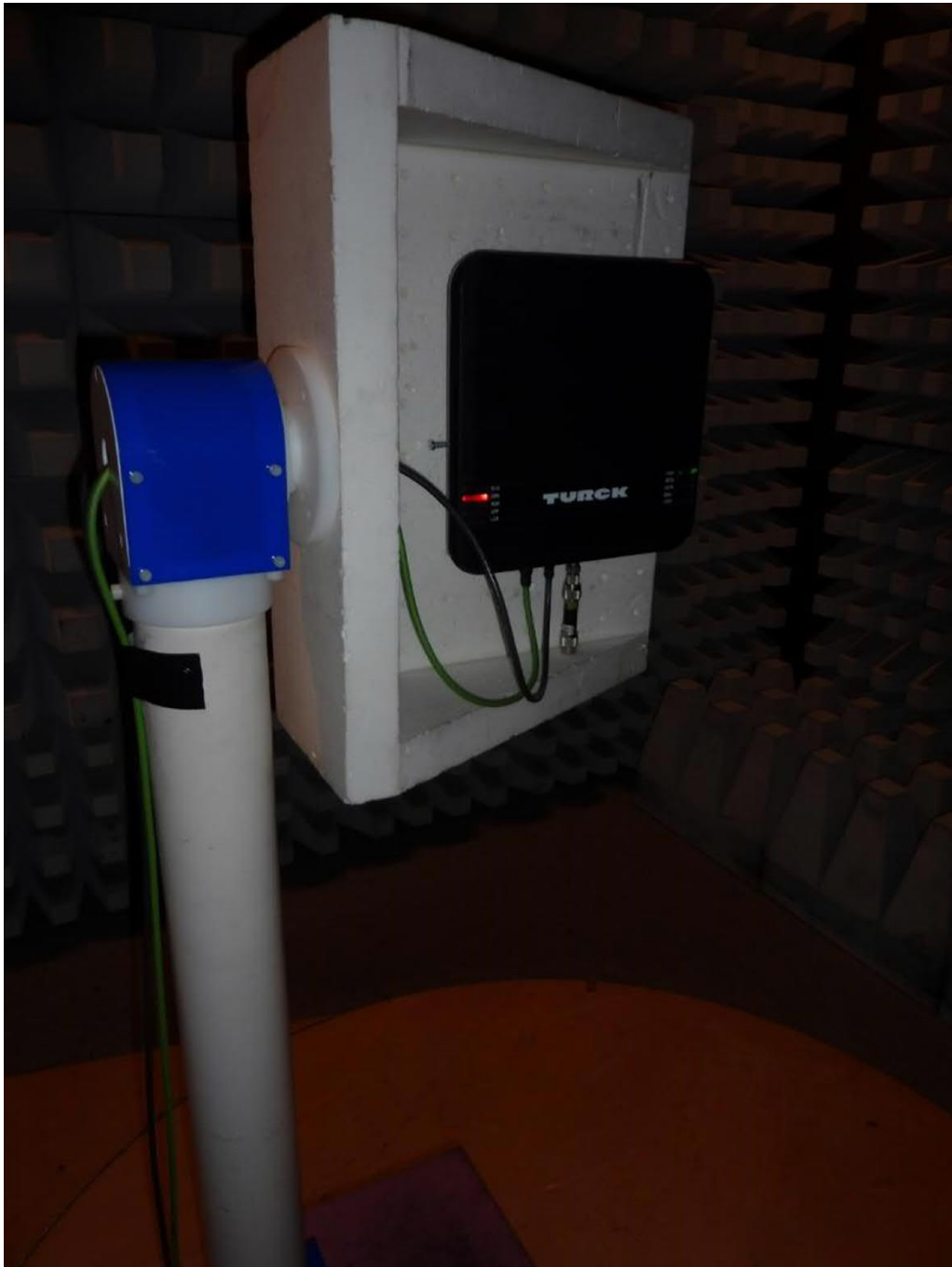
TN-UHF-Q300-NA-CDS, test setup fully anechoic chamber TX spurious emissions from 1 GHz to 10 GHz (measurement with antenna port terminated)
