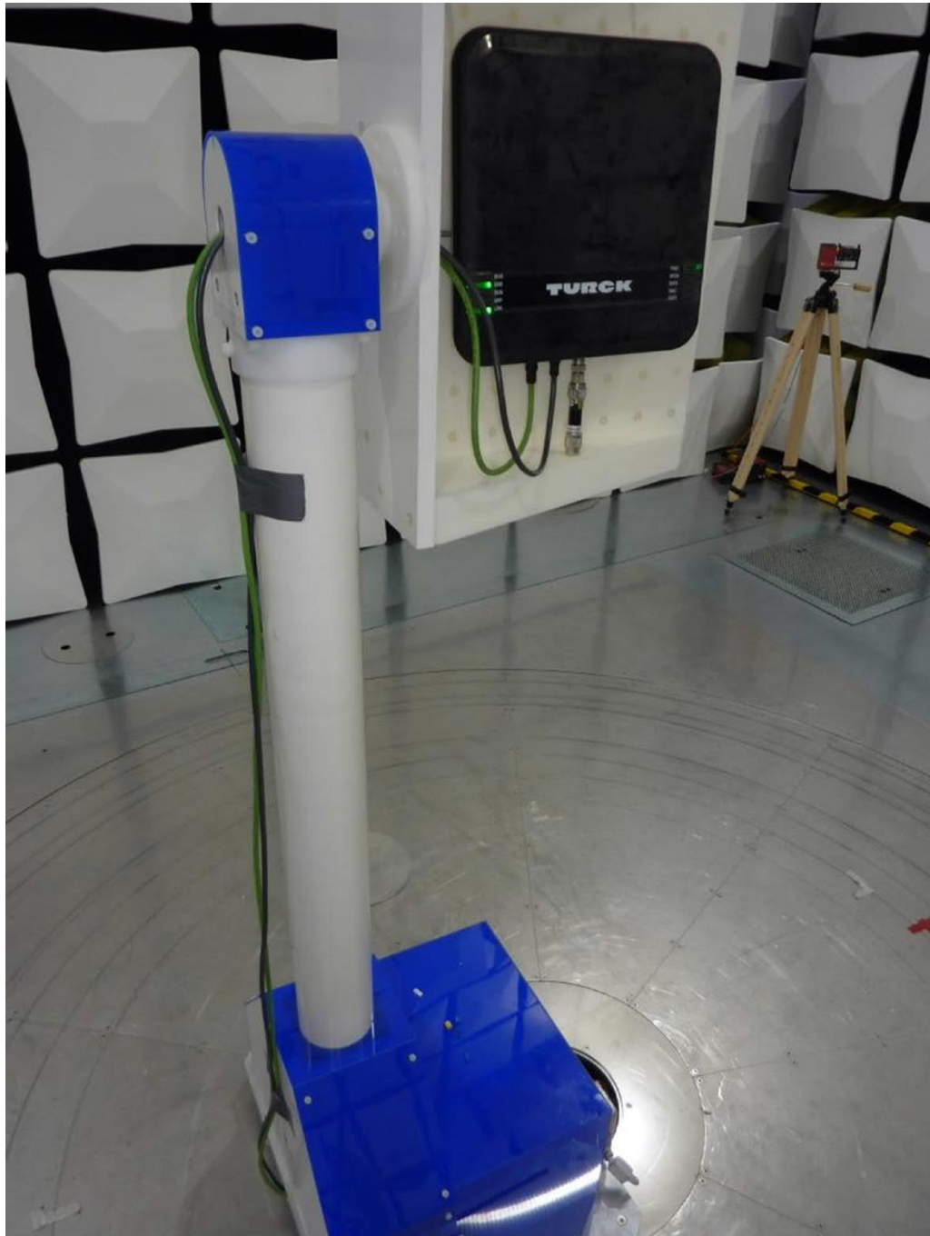
TN-UHF-Q300-NA-CDS, test setup semi anechoic chamber (measurement with antenna port terminated)
