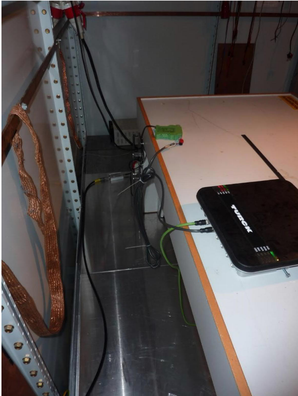
TN-UHF-Q300-NA-CDS, test setup shielded chamber (EUT DC supplied)
