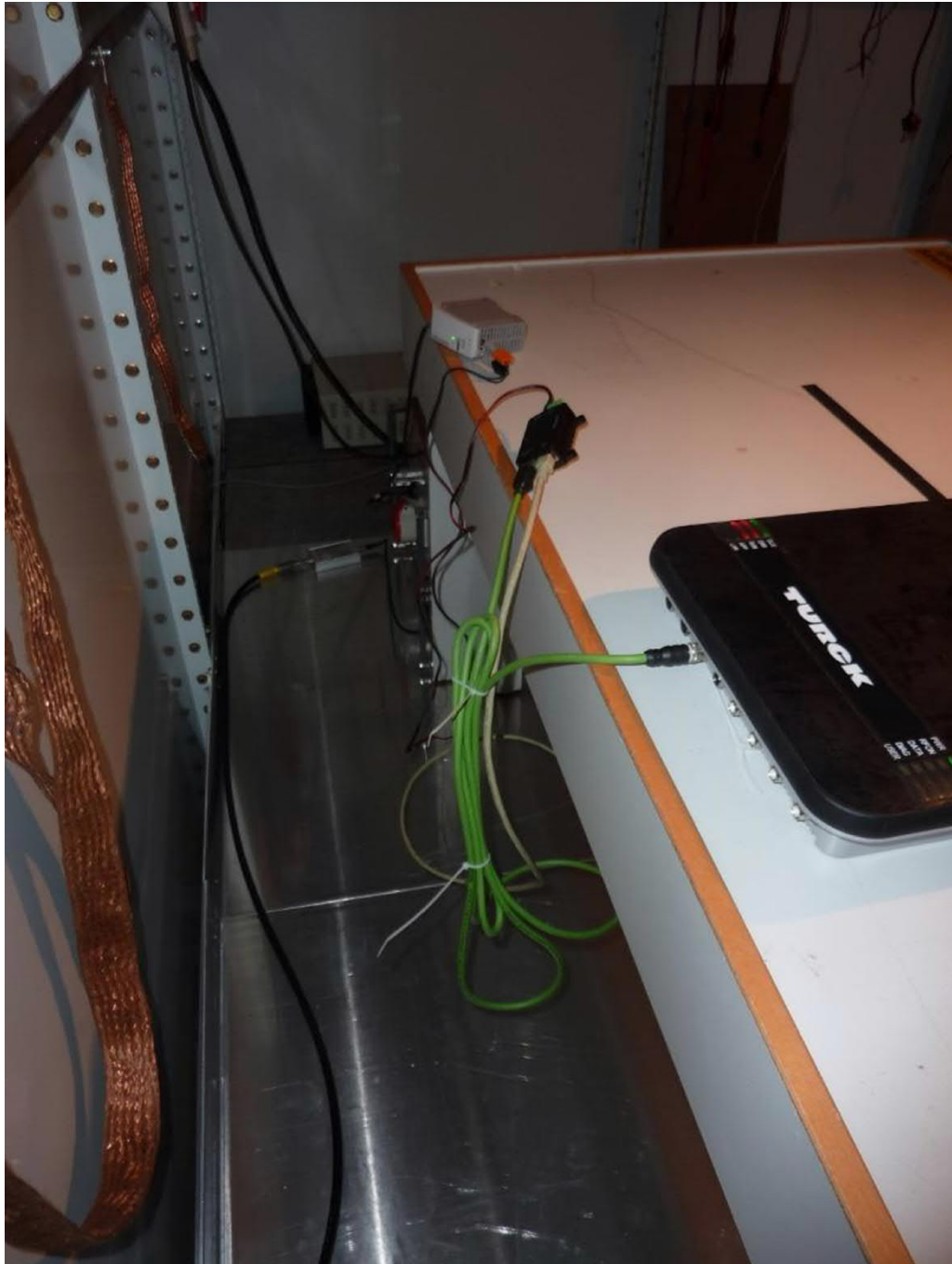
TN-UHF-Q300-NA-CDS, test setup shielded chamber (EUT PoE supplied)
