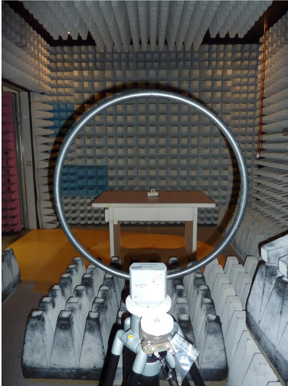
135053_13.JPG: Test setup fully anechoic chamber (H-Field)
