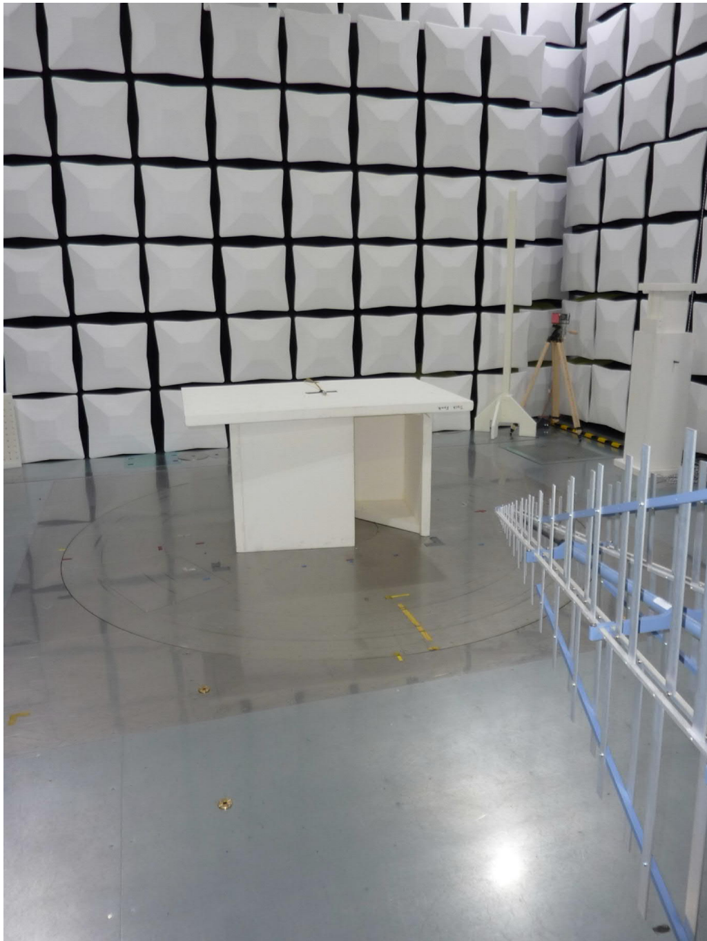
Test setup semi anechoic chamber (30 MHz to 1 GHz)
