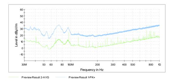
The results of the final measurement were presented on the following pages. The measured results (levels) refer to the above-mentioned standard while taking account of the specified requirements for a 3 m measuring distance.
