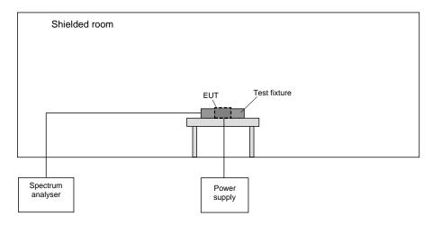
The following procedure is used for the occupied bandwidth measurement according to [1]:
