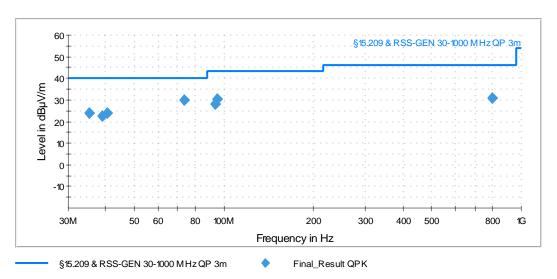
The results of the standard subsequent measurement in a semi-anechoic chamber are indicated in the table below. The limits as well as the measured results (levels) refer to the above-mentioned standard while taking account of the specified requirements for a 3 m measuring distance.
