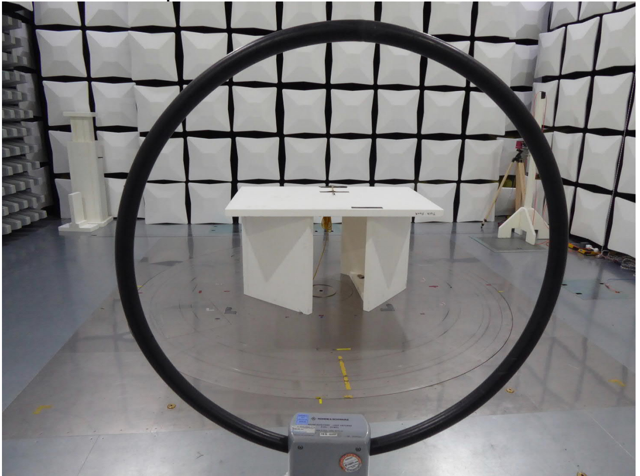
Test setup semi anechoic chamber (9 kHz to 30 MHz)
