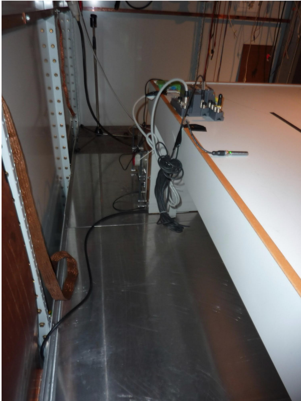
AC Mains conducted emissions test setup
