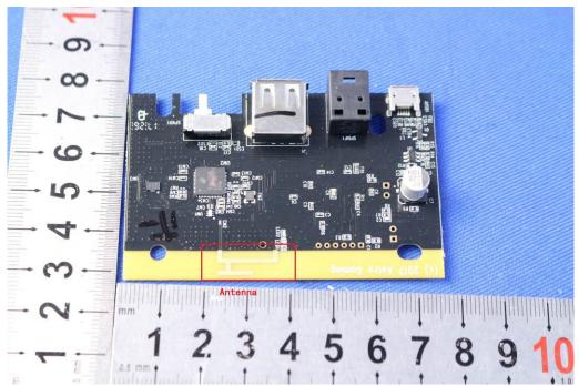
The antenna is integrated on the main PCB and no consideration of replacement. The best case gain of the antenna is 3.08dBi.
