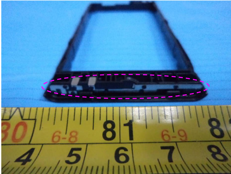
EUT – HSPA&LTE Antenna View
