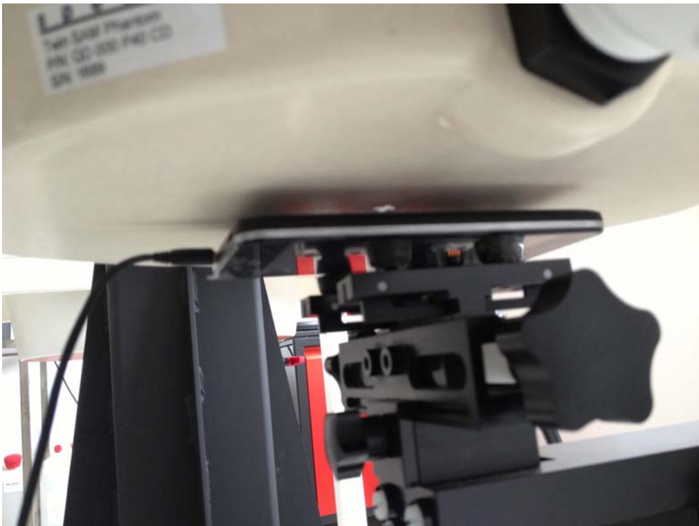
10mm Body-worn Rear (With Headset) Setup Photo
