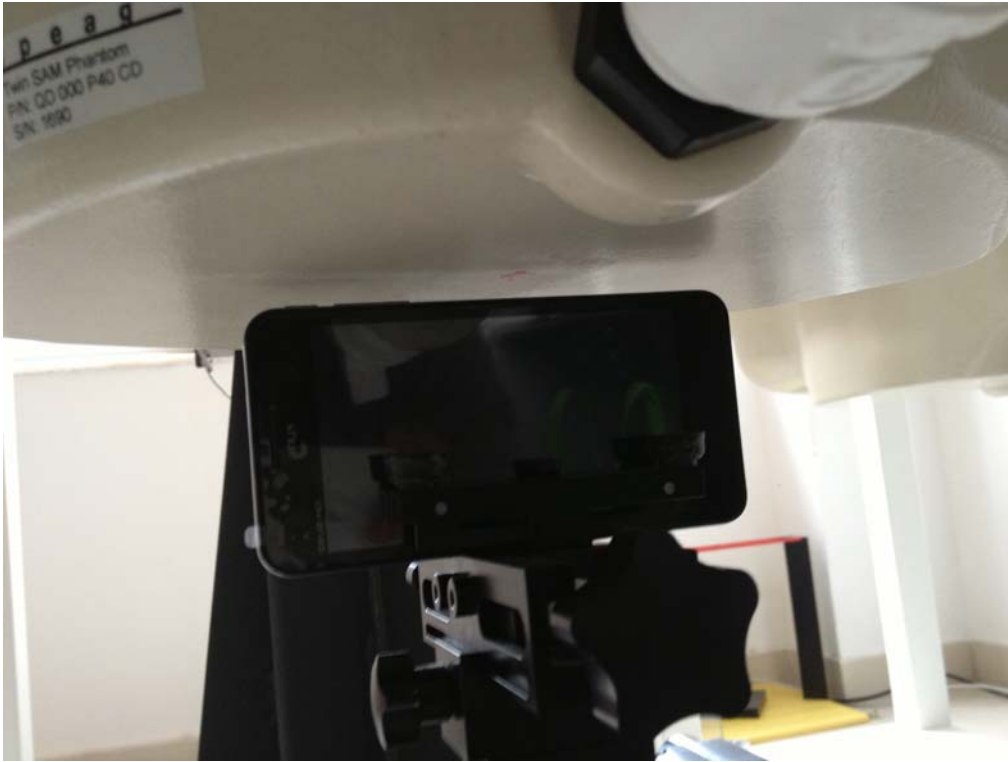
10mm Body-worn Right Side Setup Photo
