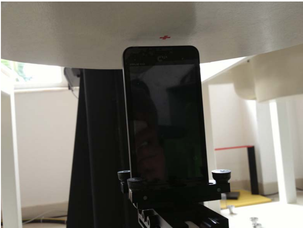
10mm Body-worn Top Side Setup Photo
