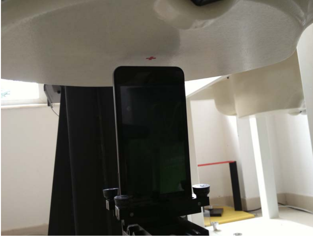
10mm Body-worn Bottom Side Setup Photo
