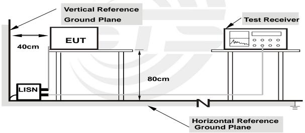
Note: 1.Support units were connected to second LISN. 2.Both of LISNs (AMN) are 80 cm from EUT and at least 80 from other units and other metal planes
