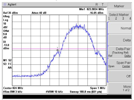
Note:Offset=Cable loss(9.5)+10log(3.2/3)=9.5+0.3=9.8 dB High Band Edge GSM 850 BAND CH 251
