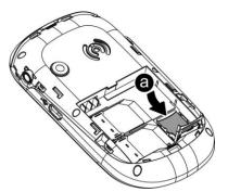
\*Note: The mobile phone does not support hot-plug function of T-FLASH in "power on" mode. Only when the mobile phone is powered off can T-FLASH be pulled out. Restart up and T-FLASH will come into effect. When using or editing files stored in the memory card, DO NOT pull out the memory card.
