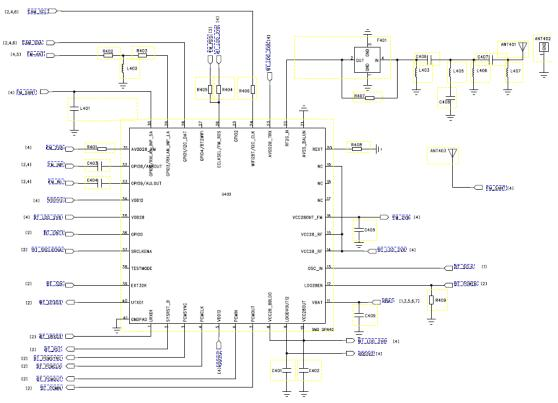
The Bluetooth overall schematic as up. MT6626 is a monolithic single chip that integrates Bluetooth V2.1+EDR and FM receiver. It can be incorporated in varieties of mobile platforms to provide Bluetooth connectivity and FM radio.
