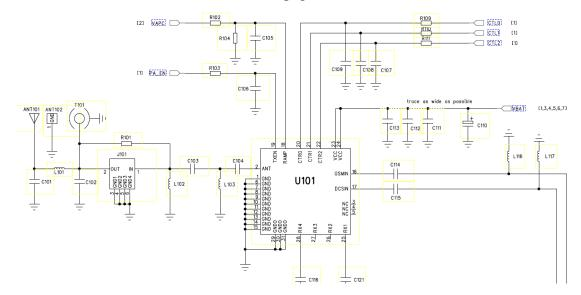
The aerial signal mobile phone received goes from antenna to RF Connector  $_{\circ}$  RF Connector, which is a special parts developed for RF test. By connecting RF cable to spectrum analyzer, you can measure RF signal.
