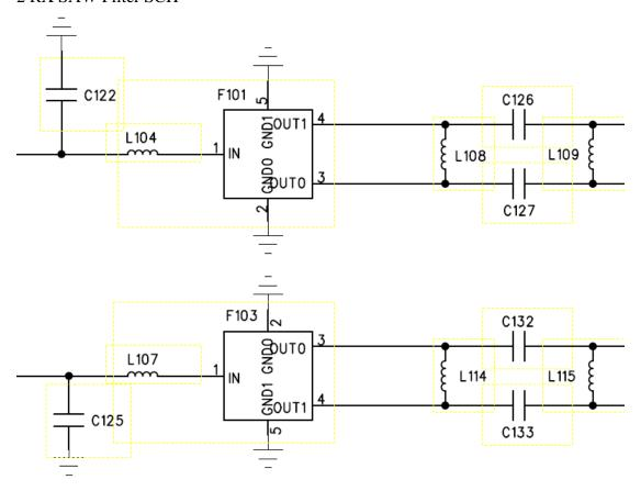
The RX signal output from RF SW, than input SAW filter .changed two difference signals
