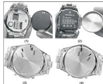
step to install the battery: from photo(1) to photo(4). step to uninstall the battery: from photo(4) to photo(1)
