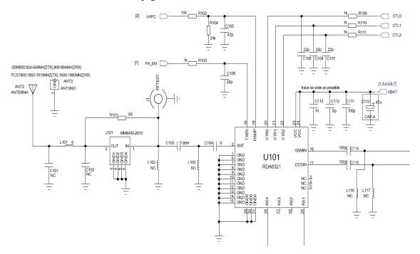
The aerial signal mobile phone received goes from GSM\_ANT to RF Connector J101 . RF Connector is a special parts developed for RF test. By connecting RF cable to spectrum analyzer, you can measure RF signal.
