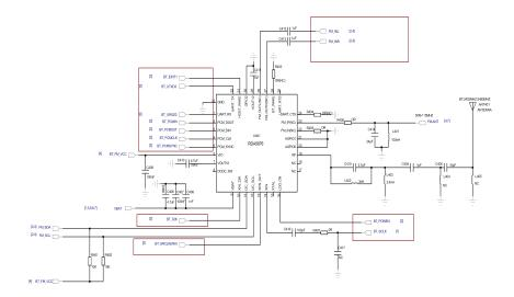
The Bluetooth overall schematic as up. RDA5876 is a highly integrated Bluetooth IC ,which is compliant with Bluetooth 2.1 + EDR specification and provides an optimal solution for data and voice application.it includes powerfull processing capabilities with rich features and a high performance transceiver ,all in a compact single package.
