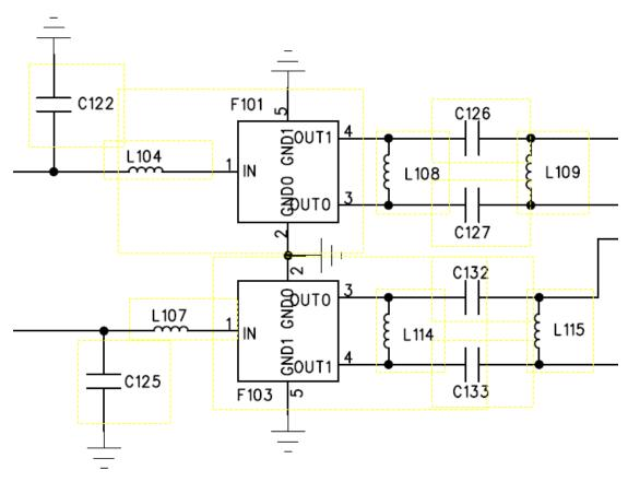
The RX signal output from RF SW, than input SAW filter .changed two difference signals in SAW filter, than input the BB transceiver of U201(MT6252).
