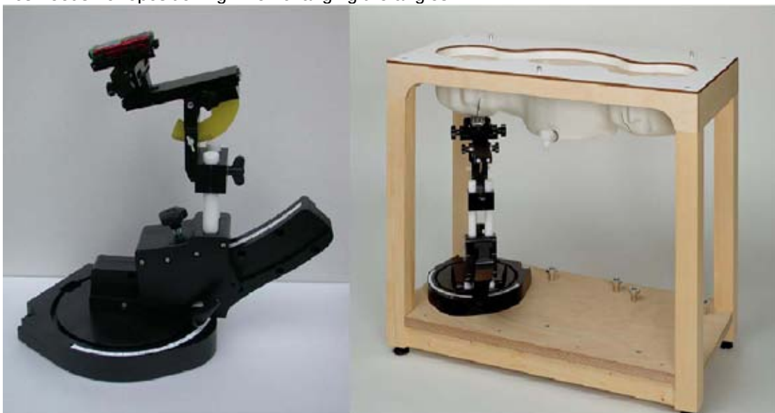
Device holder supplied by SPEAG
