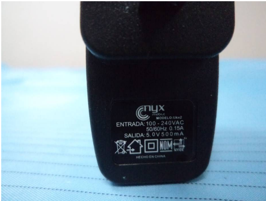
EUT – Adapter Label View
