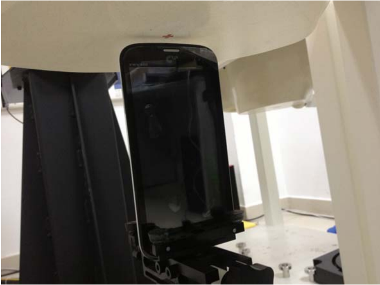
10mm Body-worn Top Side Setup Photo
