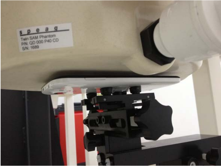
10mm Body-worn Front Side Setup Photo
