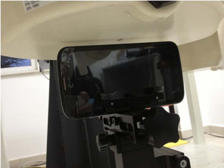
10mm Body-worn Right Side Setup Photo
