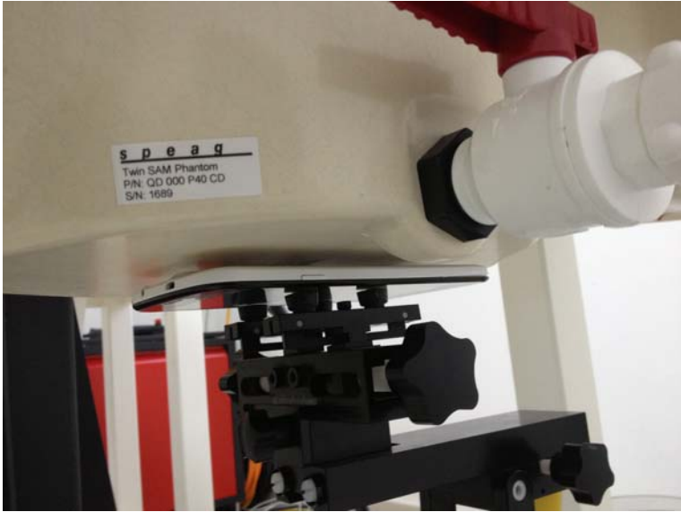
10mm Body-worn Rear Side Setup Photo
