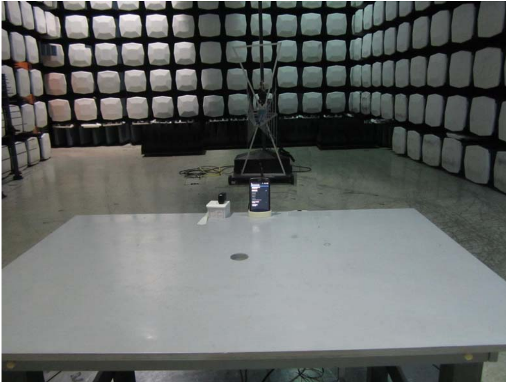
Radiated Emission (30MHz-1GHz)
