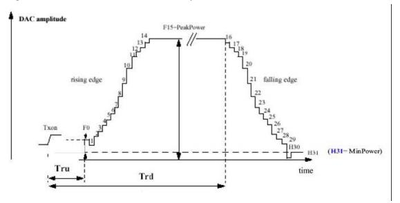
**Tru = TxTRU Default** +  $\triangle$ TRU\_P +  $\triangle$ TRU\_T **Trd = TxTRD\_NBDefault** +  $\triangle$ TRD\_P (for a normal burst). **Trd = TxTRD\_ABDefault** +  $\triangle$ TRD\_P (for an access burst).
