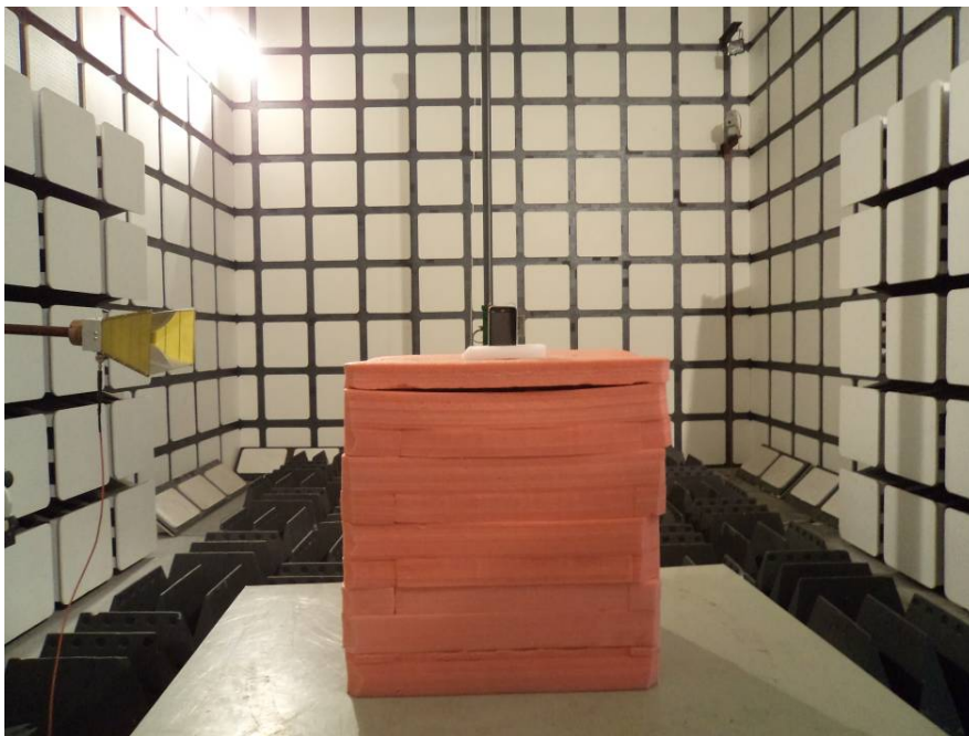
Radiated Emissions Test View (Above 1 GHz)
