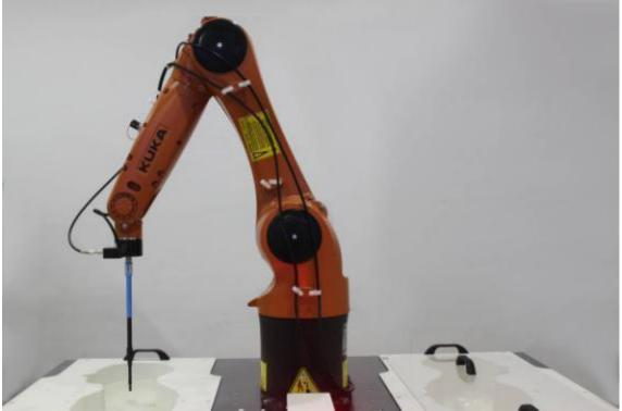
The EUT under test operating at the maximum power level is placed in the phone holder, under the phantom, which is filled with head simulating liquid. The E-Field probe measures the electric field inside the phantom. The Open SAR software computes the results to give a SAR value in a 1g or 10g mass.
