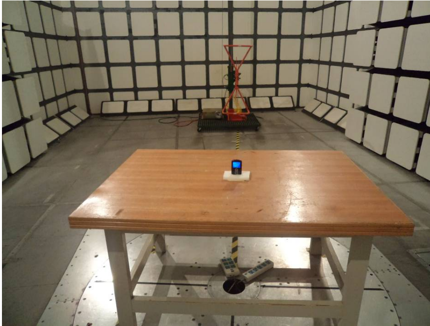
Radiated Emissions View (30-1000 MHz)
