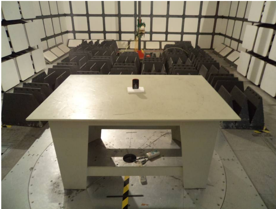
Radiated Emissions View (1-25 GHz)
