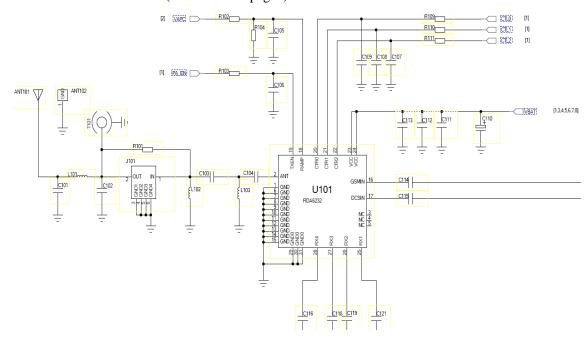
The aerial signal mobile phone received goes from antenna to RF Connector. RF Connector, which is a special parts developed for RF test. By connecting RF cable to spectrum analyzer, you can measure RF signal.
