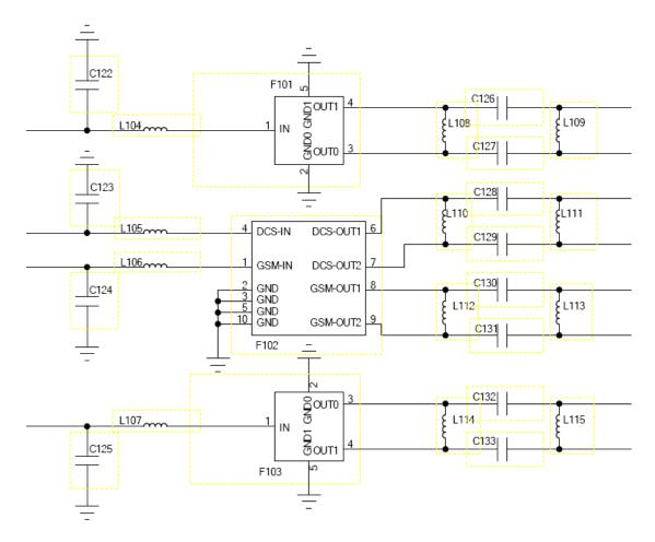
The RX signal output from RF SW, than input SAW filter .changed two difference signals in SAW filter, than input the BB transceiver of U201(MT6252)
