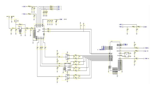
The RF overall schematic as up. It contains the TX path and RX path. The signal received from the air will be demodulated in CPU through RX SAW and Transceiver, Then the original voice signal will driver the receiver.
