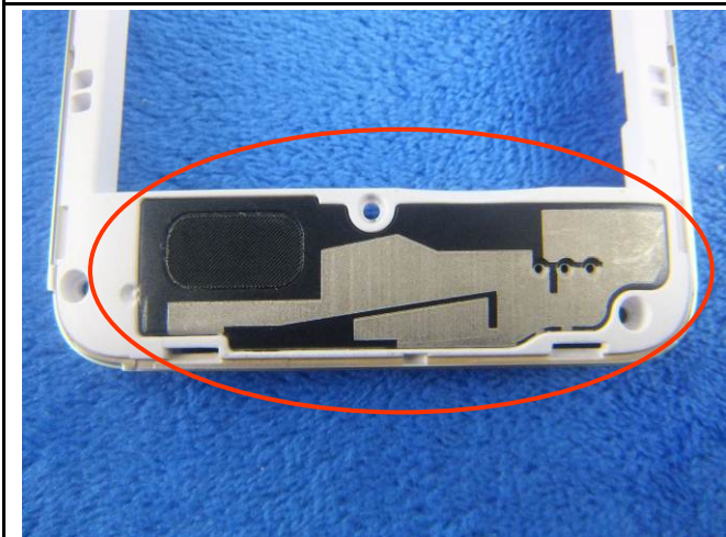
LTE Antenna View
