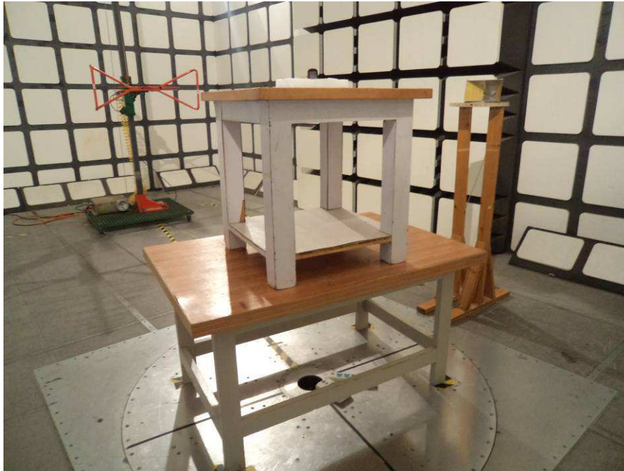
Radiated Emissions Test View (Below 1 GHz)
