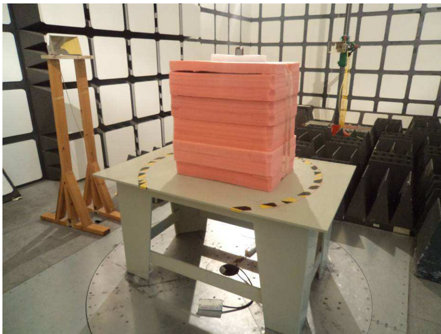
Radiated Emissions Test View (Above 1 GHz)
