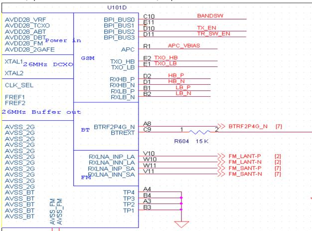
The RF overall schematic as up. It contains the TX path and RX path. The signal received from the air will be demodulated in CPU through RX SAW and Transceiver, Then the original voice signal will driver the
