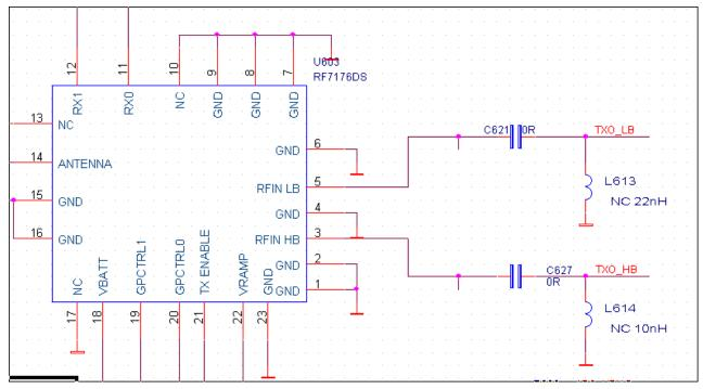
RFPA 3,5 pin connected to the CPU 101 of the E2, E1 pin
