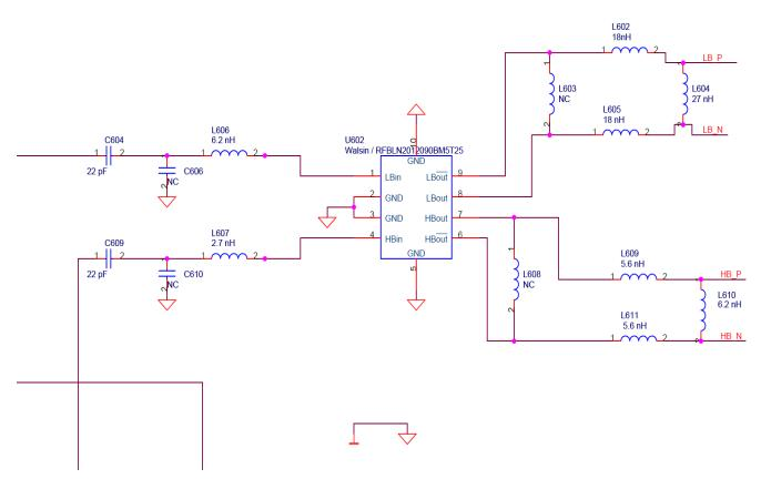
The RX signal output from RF SW, then input SAW filter .changed two difference signals in SAW filter, then input the CPU U101.
