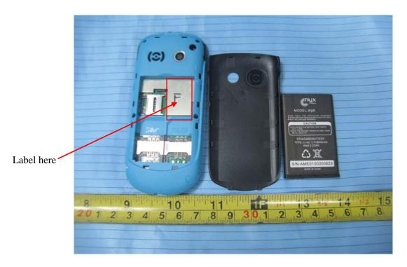
The label shown shall be permanently affixed at a conspicuous location on the device and be readily visible to the user at the time purchase (Labeling requirements per 2.925)
