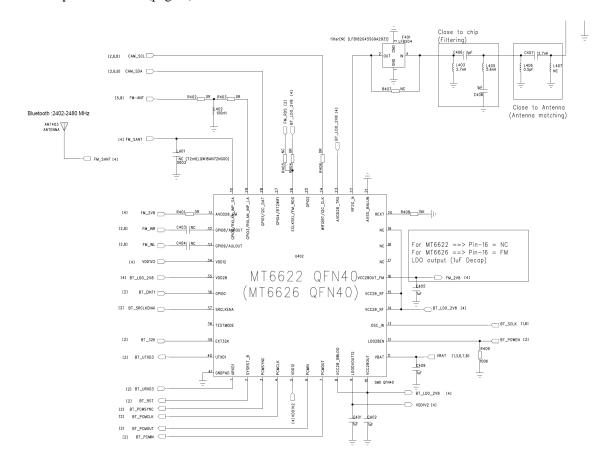
The Bluetooth overall schematic as up. MT6626 is a highly integrated Bluetooth IC, which is compliant with Bluetooth 2.1 + EDR specification and provides an optimal solution for data and voice application.it includes powerfull processing capabilities with rich features and a high performance transceiver, all in a compact single package.
