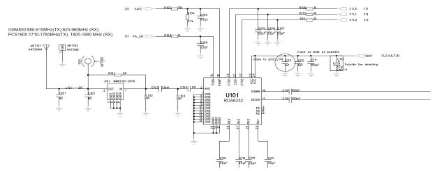
The aerial signal mobile phone received goes from antenna to RF Connector. RF Connector, which is a special parts developed for RF test. By connecting RF cable to spectrum analyzer, you can measure RF signal.
