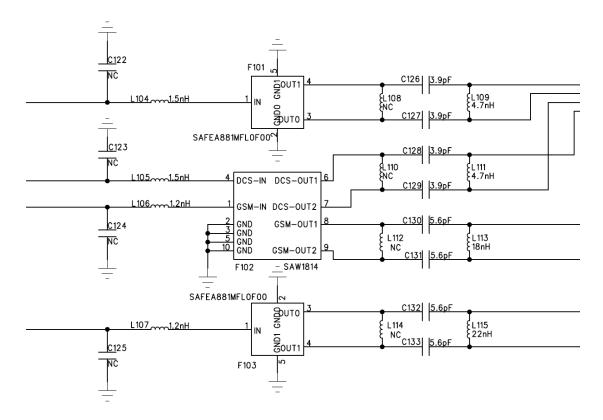
The RX signal output from RF SW, than input SAW filter .changed two difference signals in SAW filter, than input the BB transceiver of U201(MT6252)
