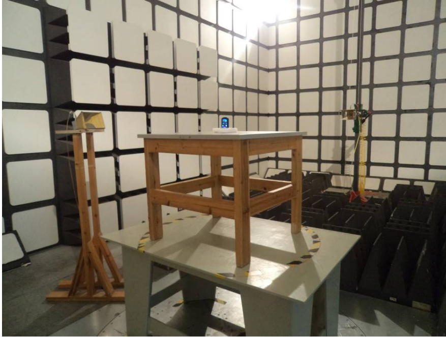
Radiated Emissions Test View
