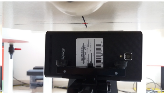
Hotspot mode - Right Side (10mm)
