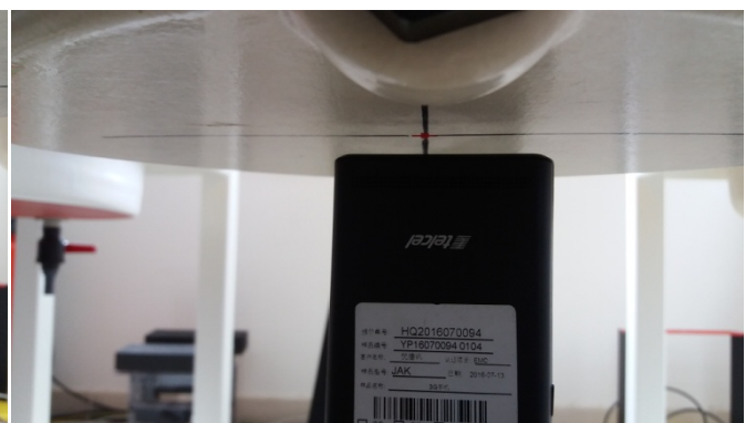
Hotspot mode - Bottom Side (10mm)
