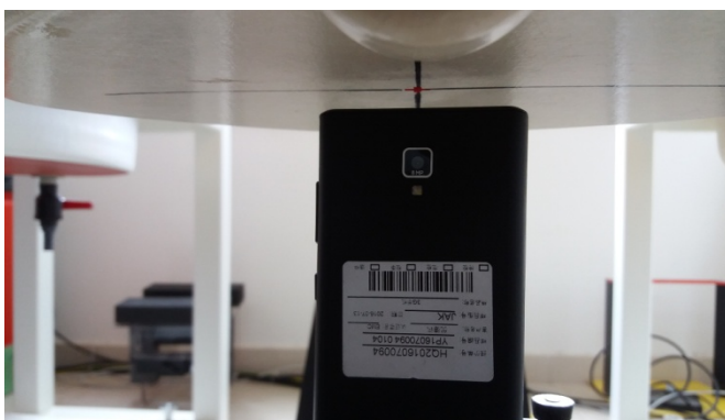
Hotspot mode - Top Side (10mm)
