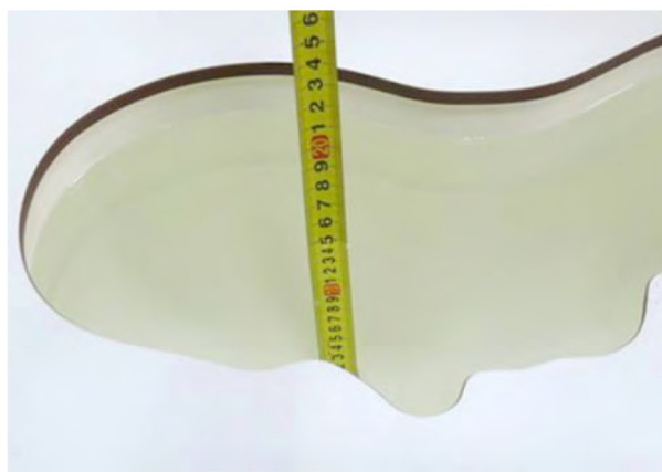
Liquid depth in the head phantom (835MHz)
