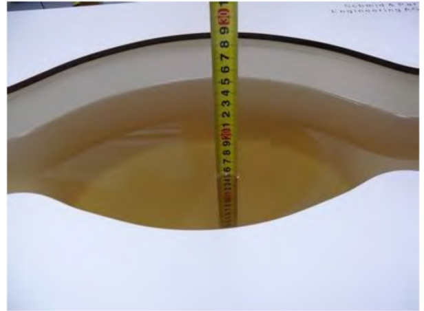
Liquid depth in the body phantom (835MHz)
