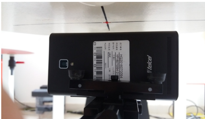
Hotspot mode - Left Side (10mm)
