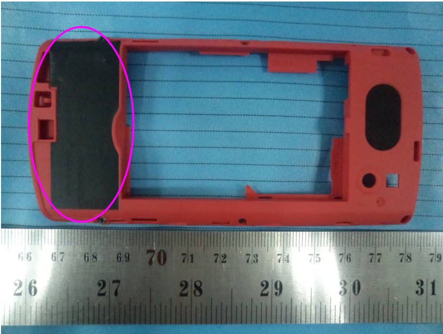
EUT – GSM/WCDMA Antenna View
