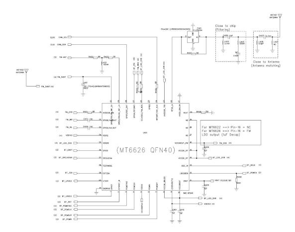
The Bluetooth overall schematic as up. MT6626 is a highly integrated Bluetooth IC ,which is compliant with Bluetooth 2.1 + EDR specification and provides an optimal solution for data and voice application. It includes powerful processing capabilities with rich features and a high performance transceiver, all in a compact single package.
