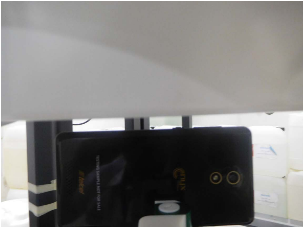
Body right side(separation distance is 10mm)
