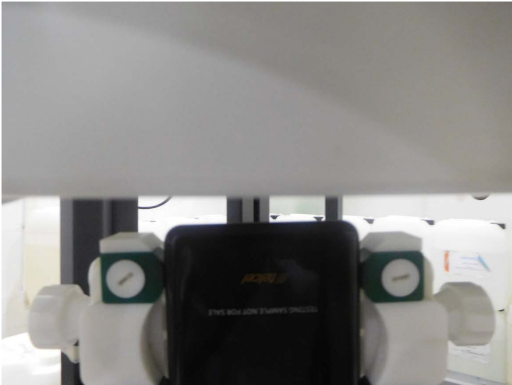
Body Bottom side(separation distance is 10mm)
