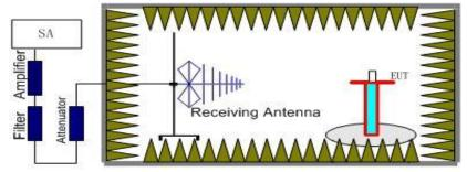
Radiated emissions measurements were made only at the upper, middle, and lower carrier frequencies It was decided that measurements at these three carrier frequencies would be sufficient to demonstrate compliance with emissions limits because it was seen that all the significant spurs occur well outside the band and no radiation was seen from a carrier in one block of any band into any of the other blocks.
