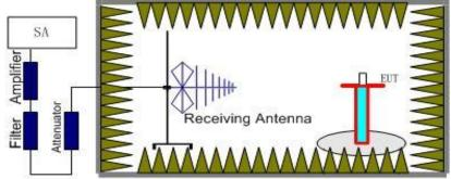
Radiated emissions measurements were made only at the upper, middle, and lower carrier frequencies It was decided that measurements at these three carrier frequencies would be sufficient to demonstrate compliance with emissions limits because it was seen that all the significant spurs occur well outside the band and no radiation was seen from a carrier in one block of any band into any of the other blocks.
