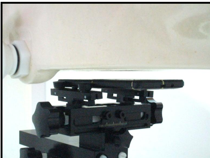
Front Face of EUT with 1.0 cm Gap
