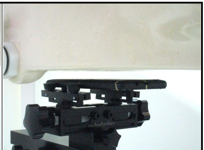
Rear Face of EUT with 1.0 cm Gap
