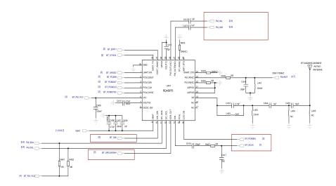
The Bluetooth overall schematic as up. RDA5875 is a highly integrated Bluetooth IC ,which is compliant with Bluetooth 2.1 + EDR specification and provides an optimal solution for data and voice application.it includes powerfull processing capabilities with rich features and a high performance transceiver ,all in a compact single package.
