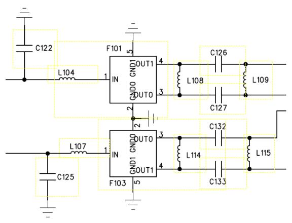
The RX signal output from RF SW, than input SAW filter .changed two difference signals in SAW filter, than input the BB transceiver of U201(MT6252C).
