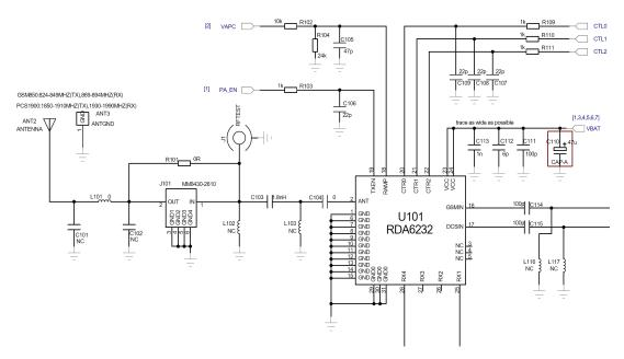
The aerial signal mobile phone received goes from GSM\_ANT to RF Connector J101 . RF Connector is a special parts developed for RF test. By connecting RF cable to spectrum analyzer, you can measure RF signal.
