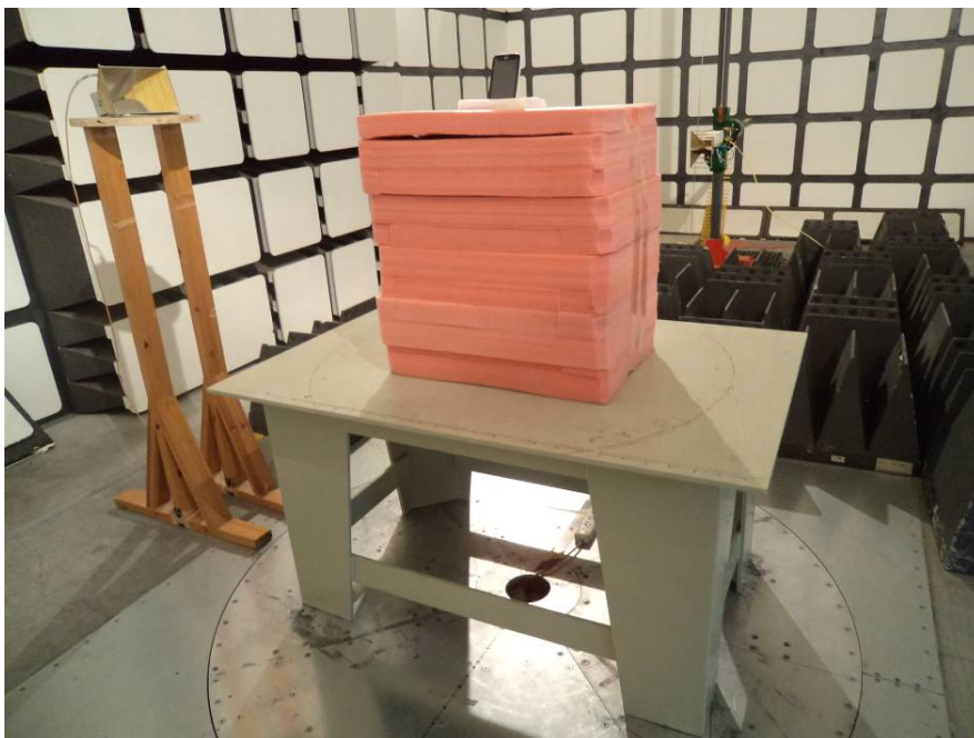
Radiated Emissions Test View (Above 1 GHz)
