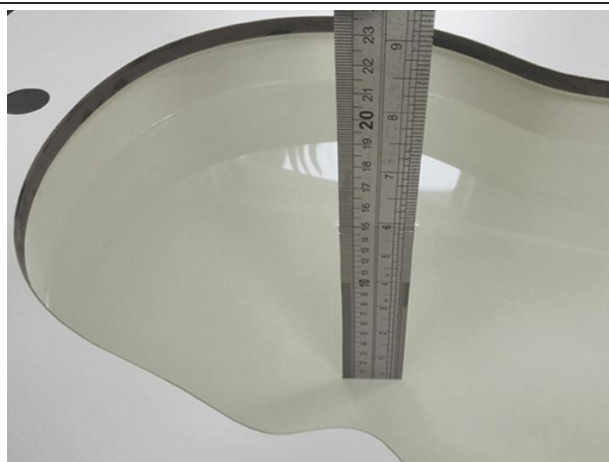
Liquid depth in the head phantom (2450MHz)
