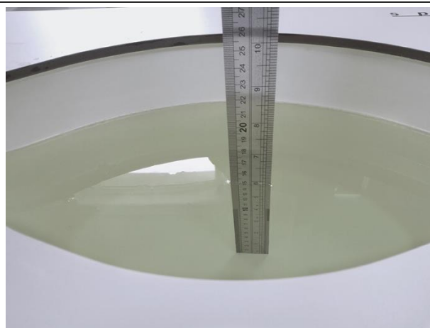
Liquid depth in the body phantom (2450MHz)
