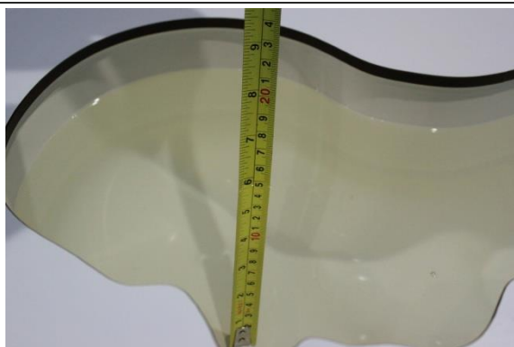
Liquid depth in the head phantom (5200MHz)
