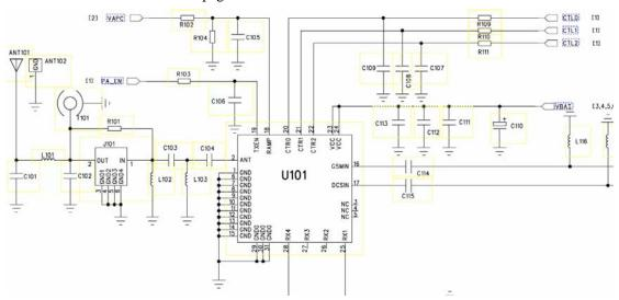
The aerial signal mobile phone received goes from GSM\_ANT to RF Connector J101 . RF Connector is a special parts developed for RF test. By connecting RF cable to spectrum analyzer, you can measure RF signal.
