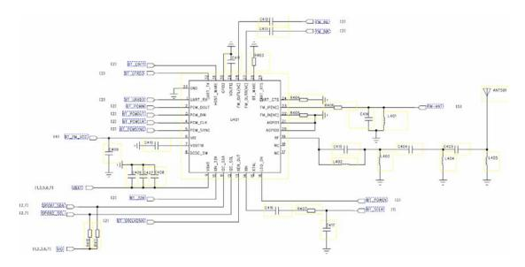
The Bluetooth overall schematic as up. RDA5876 is a highly integrated Bluetooth IC, which is compliant with Bluetooth 2.1 + EDR specification and provides an optimal solution for data and voice application.it includes powerfull processing capabilities with rich features and a high performance transceiver, all in a compact single package.
