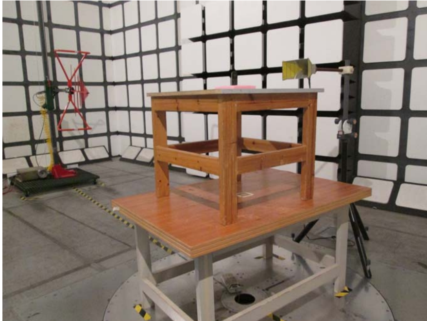
Radiated Emissions Test View (Below 1 GHz)
