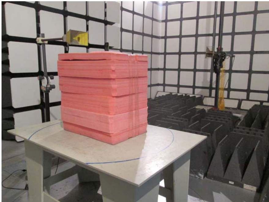
Radiated Emissions Test View (Above 1 GHz)
