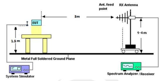
For radiated test from above 1GHz
