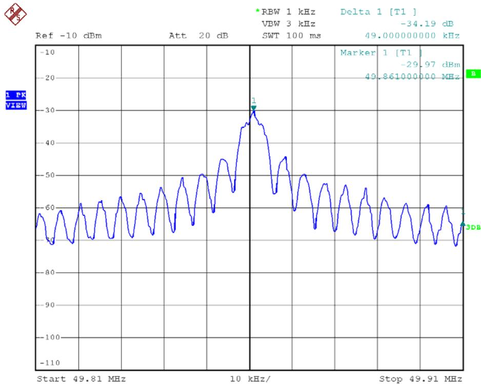
Bandwidth / Bandedge Plot – Pursuant to FCC Part 15 Section 15. 235 Requirement (Pass/Fail)
