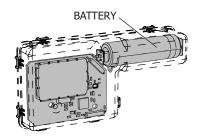
A 3.6V Lithium battery is integrated directly into the dispenser telemetry module as a non-replaceable power source.
