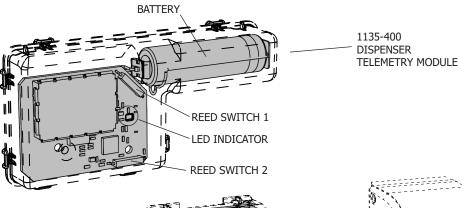
The Telemetry module is installed into the dispenser mechanism, along with the activation magnet.
