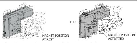
To aid installation a Light Emitting Diode (LED) is provided. To activate installation mode hold the mechanism in the activated position, as shown above, for approximately 5 seconds. Provided a working Wireless basestation is in radio range the LED will flash slowly 5 times.
