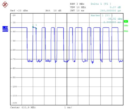
Average Factor Plot – Pursuant to FCC Part 15 Section 15. 231(e) Requirement (Pass/Fail)
