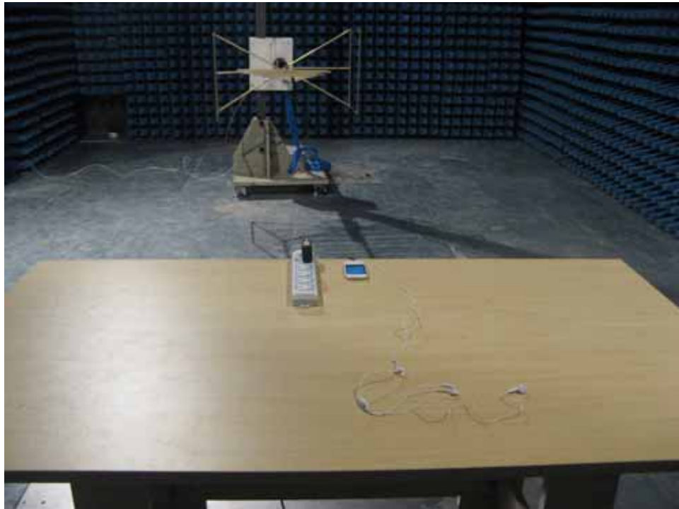
FCC RADIATED EMISSION TEST SETUP FOR CHARGER MODE
