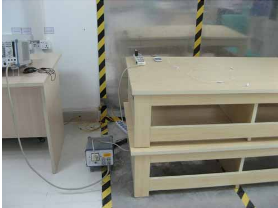
FCC RADIATED EMISSION TEST SETUP FOR PC MODE
