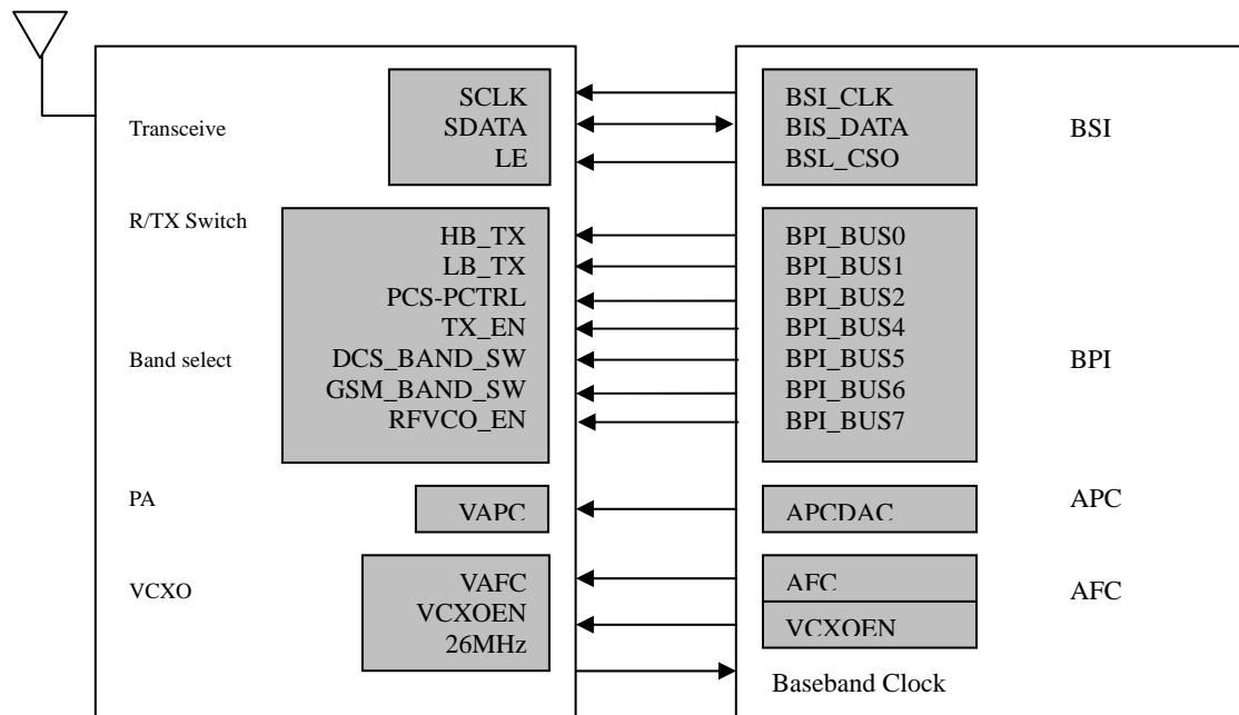
**GSM RF and BB interface diagram**
