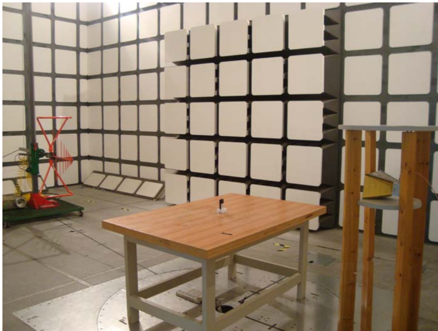
Below 1GHz: Spurious Radiated Emissions - Rear View
