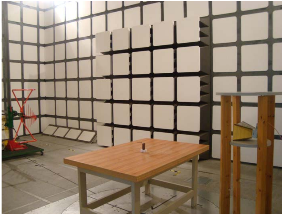
Below 1GHz: Spurious Radiated Emissions - Front View
