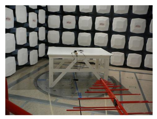
Radiated Emission below 1 GHz Rear View (Integrated ceramic chip Antenna)
