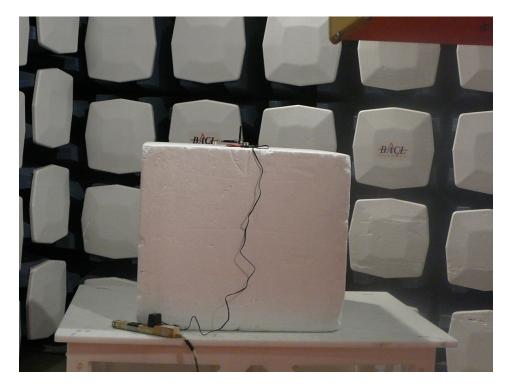
Radiated Emission above 1 GHz Rear View (Dipole Antenna)
