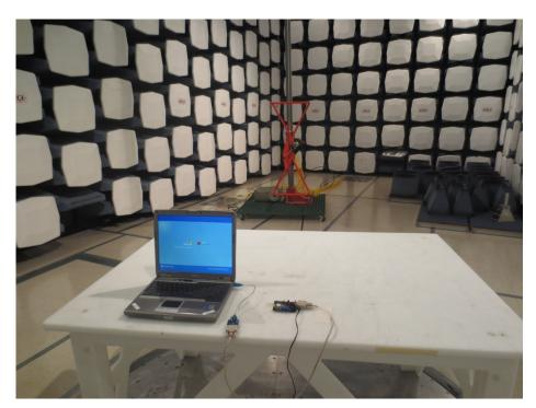
7.2 Radiated Emission below 1 GHz Rear View at 3m
