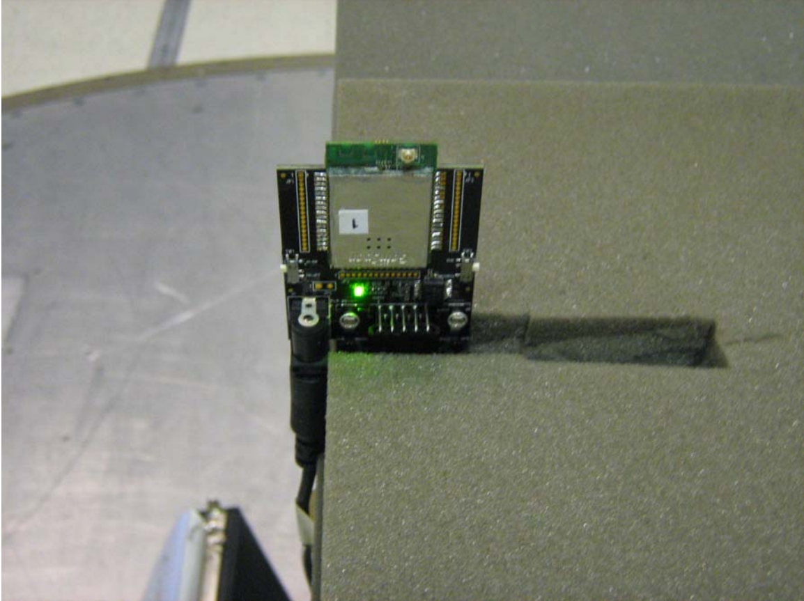
Figure 9: Radiated Emission Setup on Z-Axis
