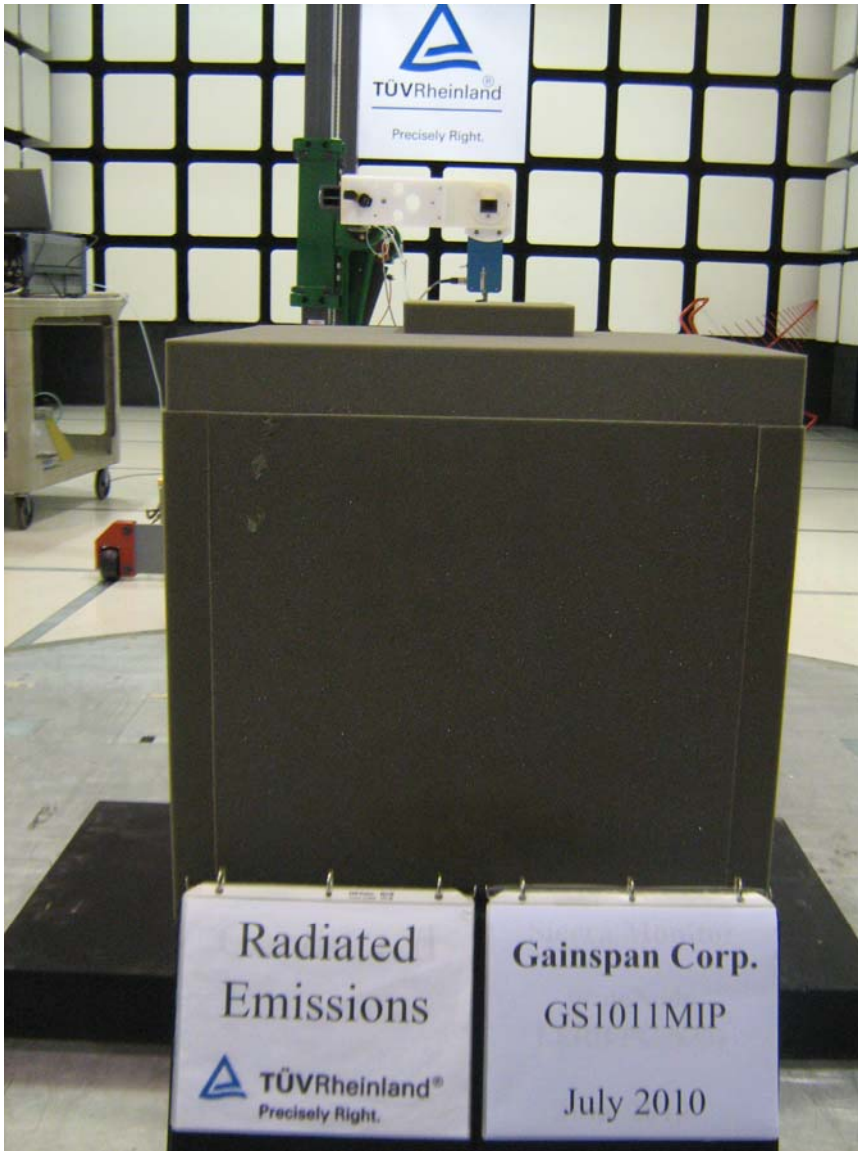
Figure 6: Test Setup for 18 GHz to 26GHz (Rear View)
